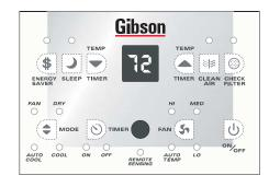
**Note:** Tap or hold either up ( $\bigstar$ ) or down ( $\checkmark$ ) button until the desired temperature is seen on the display. This temperature will be automatically maintained anywhere between 62°F (17°C) and 86°F (30°C) for cooling mode. If you want the display to read the a ctual room temperature. See "To Operate on Fan Only" section on Page 8.
